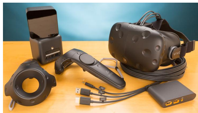
Fig. 3: The HTC Vive HMD, along with the handheld controllers and the tracking cubes. The controllers allow interaction with the sub-assemblies of the vessel model, as well as graphical-interface specific interactions (menus etc). The tracking cubes serve as reference points for the HMDs, to determine user location and gaze orientation.
