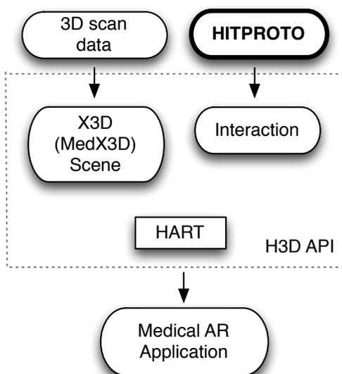
Figure 3: Due to its reliance on standards the HITPROTO toolkit can be combined with popular APIs to produce AR scenarios (such as medical AR with the use of 3D scan datasets), allowing the developer to quickly prototype haptic interactions with those objects.
