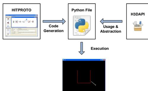
Figure 2: HITPROTO toolkit architecture. Haptic interactions are modelled using HITPROTO. The produced interactions, (saved in Python) are interpreted by H3DAPI and can be integrated in larger systems
