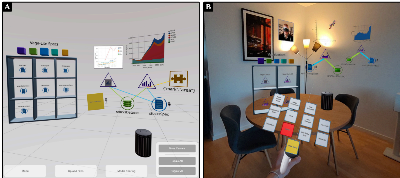
Fig. 2: DashSpace on Desktop and HMD. (A) The bookshelf showing available Vega-Lite specs in the library. A 2D and 2.5D visualization connected to the same dataset and spec; the latter is connected to a snippet that changes the mark type. A sticky note is visible in the center. (B) The bookshelf shows available visualization types as well as a 3D Optomancy and a 2.5D Vega-Lite visualization. The controller menu is visible in the foreground; in the background, a virtual image has been placed on the wall besides the physical one.
