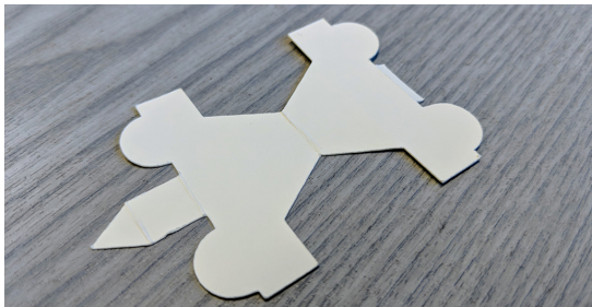
Figure 6: Simplified car model, that can be assembled without glue. Cut by the Cricut Explore Air 2 cutter.
