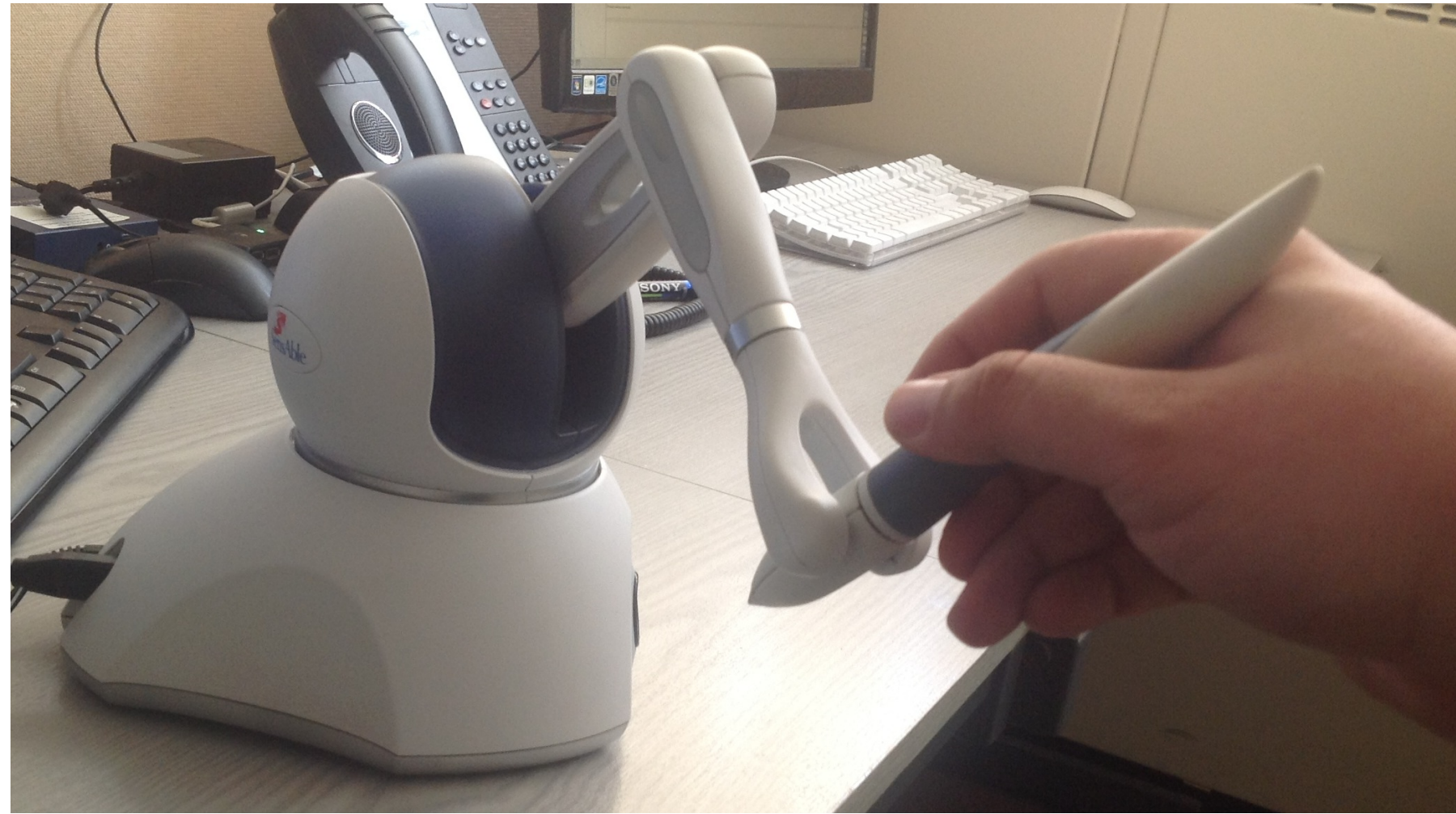
The Geomagic Touch (PHANToM Omni)
